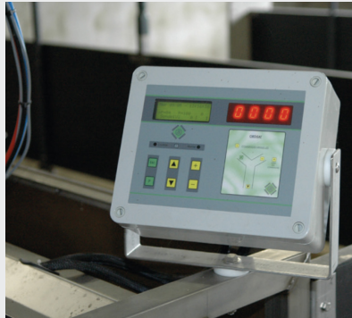
WEIGHING SYSTEM ON THE TOP OF ORDISAT CONCEPT (CONVENIENT ACCESS)
