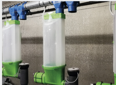
SCREW DOSING FOR FLOUR AND GRANULES WITH FLOW CONTROL SYSTEM
