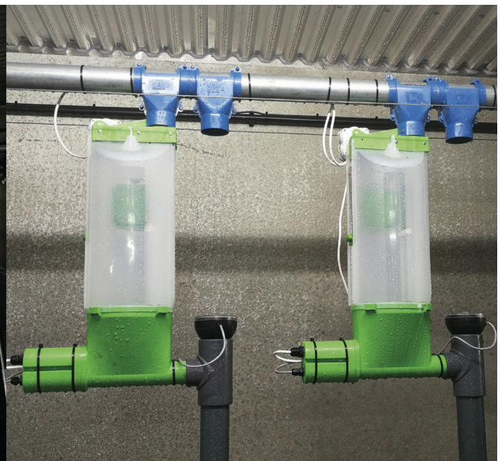
SCREW DOSING FOR FLOUR AND GRANULES WITH FLOW CONTROL SYSTEM
