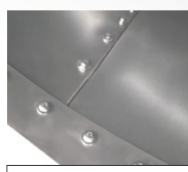
flat head screw to avoid obstructions
